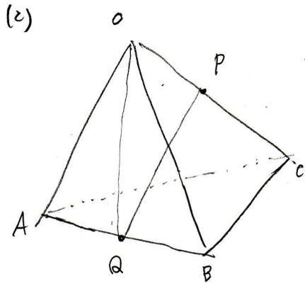
$$\begin{aligned} \vec{OP} &= t\vec{OC} = (3t, 0, -3t) \\ \vec{OQ} &= \vec{OA} + s\vec{AB} & \vec{AB} &= (-3, 0, -3) \\ &= (3, 3, 0) + (-3s, 0, -3s) \\ &= (3-3s, 3, -3s) \\ |\vec{PQ}|^2 &= (3t-3+3s)^2 + 3^2 + (-3t+3s)^2 \\ &= 18t^2 - 18t + 18s^2 - 18s + 18 \\ &= 18(t - \frac{1}{2})^2 + 18(s - \frac{1}{2})^2 + 9 \end{aligned}$$
